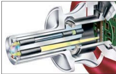
All measuring components are in one solid CORE-optics module. The patented CORE-optics is mechanically isolated from the influence of external forces and vibrations. The CORE-optics contains no mechanical adjustments.
