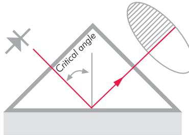
A digital CCD-camera detects the optical image and the shadow line. The camera transforms the optical image point-by-point to an electrical signal. The exact shadow line position is located and the refractive index  $n_D$  is determined.
